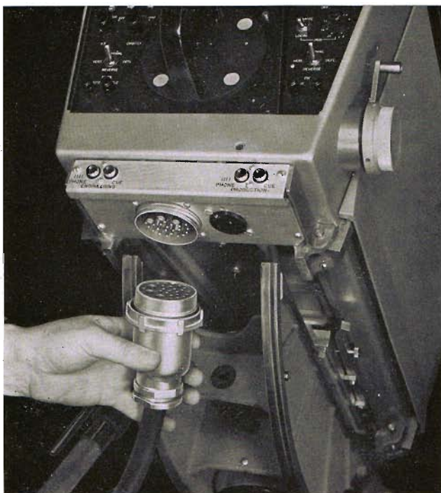
TK-60A uses standard camera cable and connectors for complete interchangeability with existing equipment.
